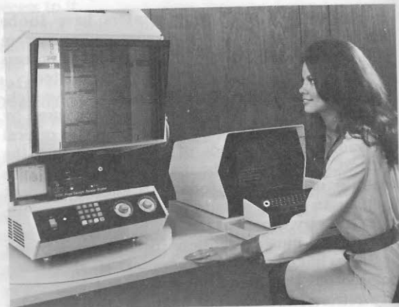
The 3M Microdisc system is a random access retrieval system which combines the high density storage efficiency of 16mm microfilm cartridges with the rapid inquiry capability to an index stored on a magnetic disc.
